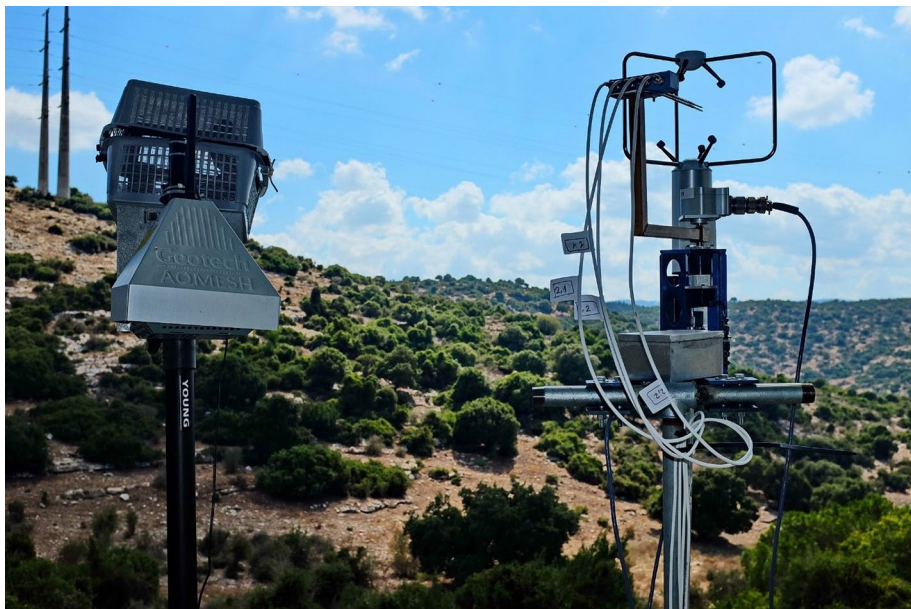
Fig. 1 Measuring instruments: on the left side of the image are the AQMesh (pyramid shaped device) and the laser particle counter (inside the plastic cage); on the right side of the image is the combo including ultrasonic anemometer and the two X-shaped HF probes
