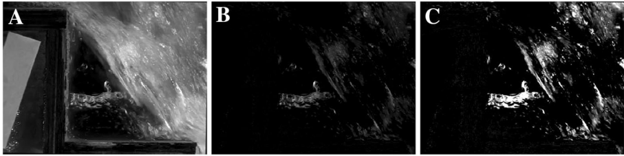
Fig. 3 Image pre-processing steps; flow direction from left to right; step-cavity 5; Re = 1.3 \times 10^5 ; d_c/h = 0.5 . a (Left) original image. b (Middle) background subtraction. c (Right) contrast enhancement
