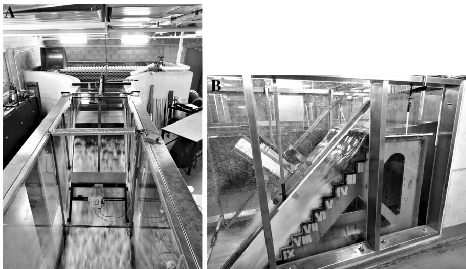
Fig. 2 Physical model of the stepped spillway; d_c/h = 0.8 ; Re = 2.7 \times 10^5 ; \theta = 45^\circ . a (Left) top view; inlet basin, side-wall convergent and stepped chute. b (Right) lateral view; flow direction from right to left
