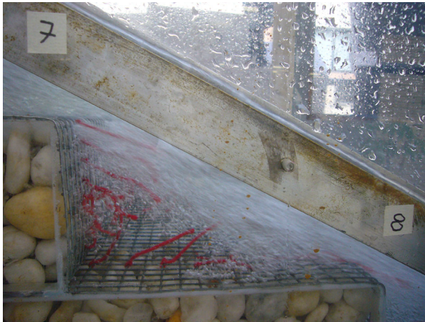
Fig. 5 Cavity flow pattern in a skimming flow on gabion stepped weir - Flow conditions: step cavity 7–8, Q = 0.068\text{m}^3/\text{s} , d_c/h = 1.20 , Re = 5.2 \times 10^5 - Note the clear water core in the step cavity
