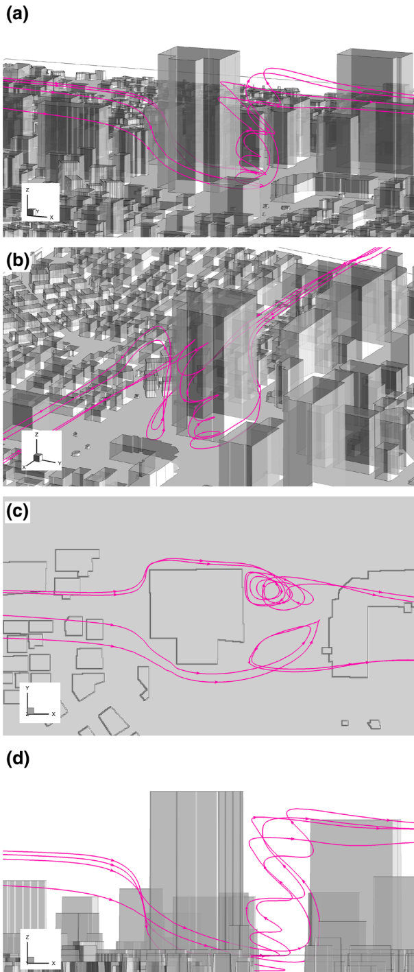
Fig. 10 Streamlines passing around tall buildings for the wind direction of 0^\circ : perspective views in a transverse and b streamwise directions; c top view; d side view
