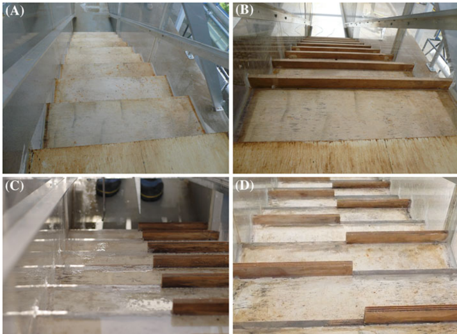
Fig. 3 Photographs of the stepped configurations including in-line and staggered stepped arrangements ( Bottom ) View from upstream looking downstream ( a, Left ) Flat stepped arrangement ( b, Right ) Pooled stepped arrangement ( c, Left ) In-line stepped arrangement ( d, Right ) Staggered stepped arrangement
