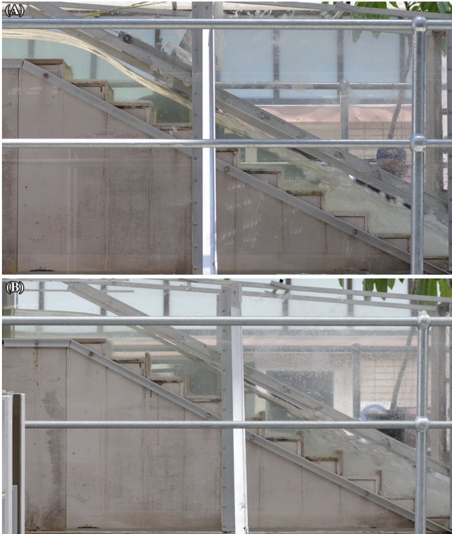
Fig. 4 Skimming flow regime on flat and pooled stepped spillways. a Flat steps, Q = 0.114\text{m}^3/\text{s} , d_c/h = 1.7 , Re = 8.8 \times 10^5 . b Pooled steps, Q = 0.100\text{m}^3/\text{s} , d_c/h = 1.56 , Re = 7.7 \times 10^5
