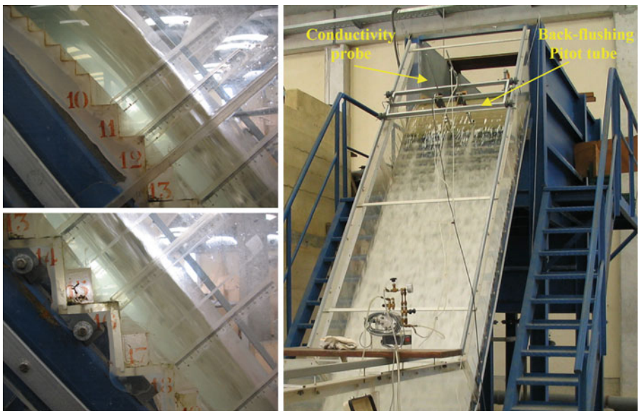
Fig. 2 Experimental flume and instrumentation (conductivity probe and back-flushing Pitot tube) at LNEC
