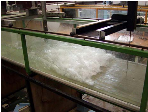
Fig. 4 Hydraulic jump in the experimental facility at the University of Queensland (flow from right to left, Fr = 5.1 )
