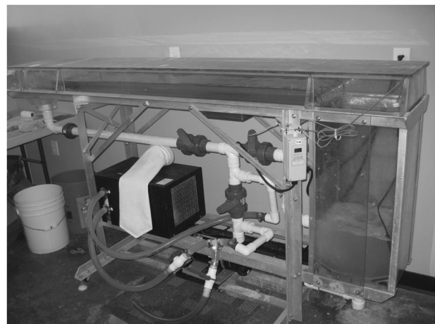
Fig. 1 Picture of laboratory flume used to conduct experiments
