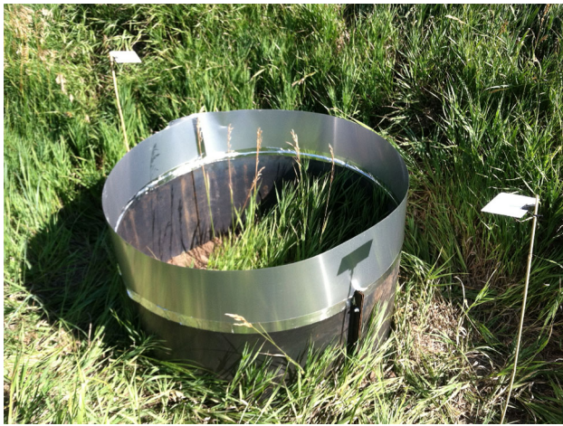
Fig. 2 Example of the open-top metal enclosures and paper samplers deployed to fields prior to treatment with Headline AMP Fungicide. Figure depicts an enclosure in the potential drift area
