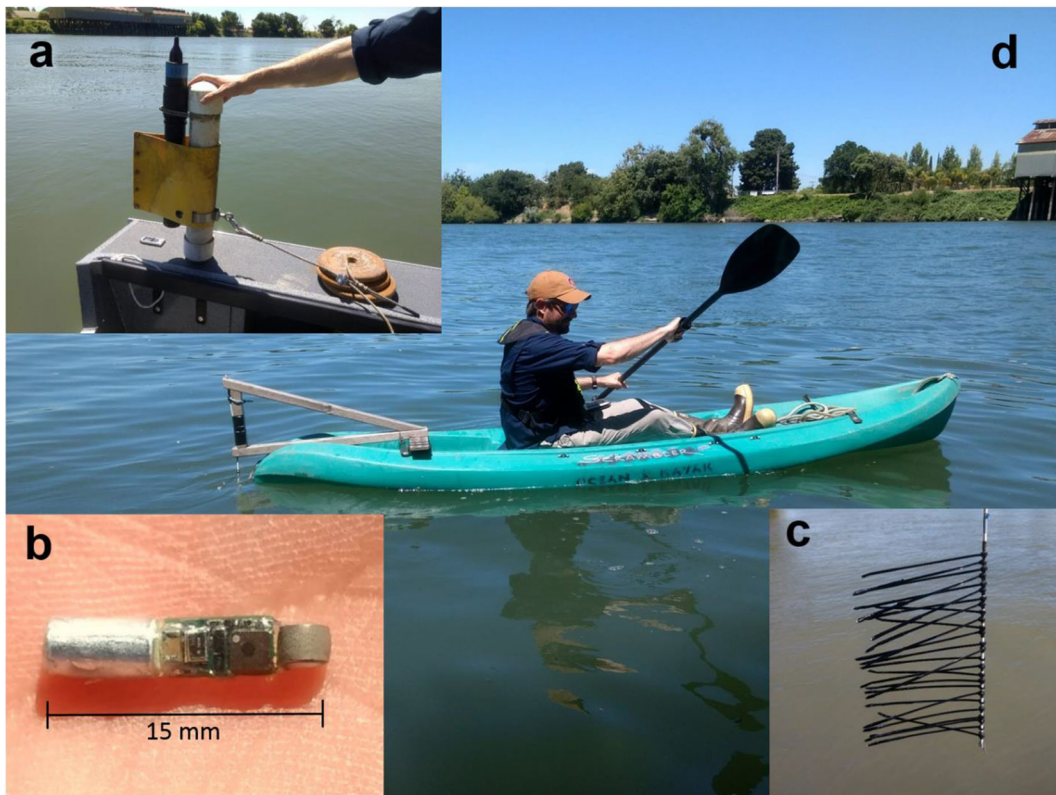
Fig. 2 a JSATS receiver with buoyancy tube, stabilizing fin and 18 kg weight. b JSATS pin transmitter (tag) with dimensions of 15 mm length \times 3.4 mm diameter and weight of 0.22 g. c
