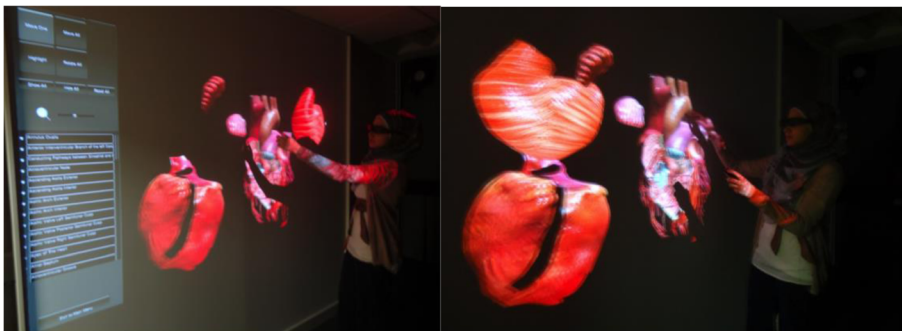
Fig. 1 Remote manipulation of 3D data in semi-immersive environment (projection wall and active stereo 3D glasses). (Glasgow Caledonian University/United Kingdom) (Adapted from (Falah et al. 2015))
