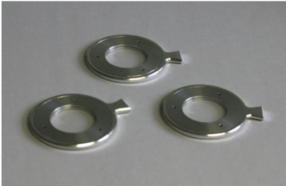
Fig. 2 The LEE and Luminit filters were mounted in aluminum rings for insertion into a trial frame
