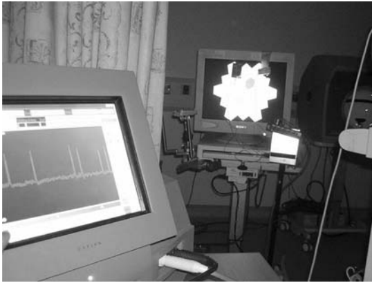
Fig. 2 Set up for recording the sequences. Nineteen segment display with photodiodes (right) and flash sequence captured (left)
