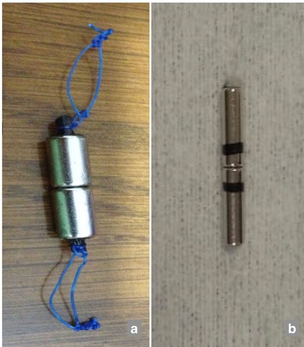
Fig. 1 Magnet types used in the study. a Coupled N35 magnets with a pit at the tip of the magnet that enables 2–3 cm fishline (or 2/0 prolene suture thread) attachment with superglue. b Coupled hole-through N52 magnets marked at the opposite poles with a board marker
