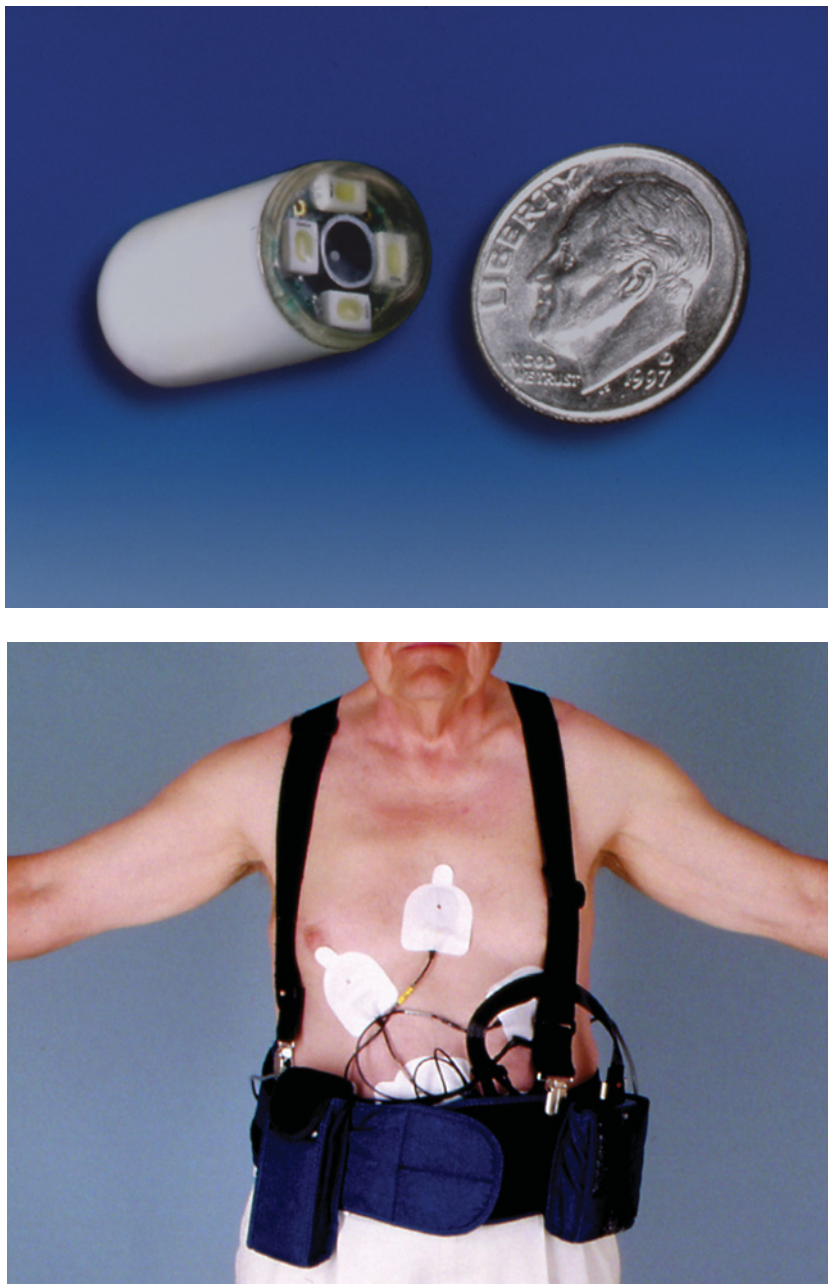
Fig 1. (A) The capsule endoscope is small enough to be swallowed easily. (B) The sensor array attaches to the data recorder carried on a belt around the patient's waist.
