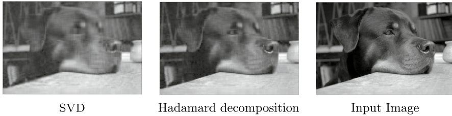
Fig. 2 Example: Hadamard decomposition and svd in the task of image compression. Both the Hadamard decomposition and the svd use 20 basis vectors for compression. Although the Hadamard decomposition and the svd rely on the same total number of vectors to represent the input image, the reconstruction provided by the Hadamard decomposition is of higher quality. In particular, the Hadamard decomposition incurs a total sum of squared errors lower than the svd by 43%
