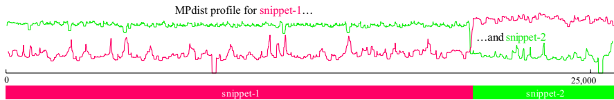
Fig. 19 (Top) The profiles that were used to compute the top two snippets. (Bottom) It is from these curves that we obtain the “regime bar,” which tells us which snippet explains which region of data
