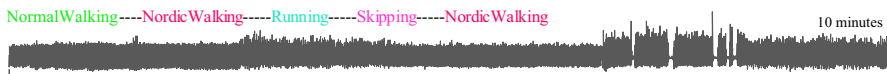
Fig. 20 A 10-min region of behavior from the PAMAP dataset (Reiss and Stricker 2012). The data is the Y-axis acceleration from a chest-worn sensor. In this dataset the ground truth is available from careful annotations made at the time
