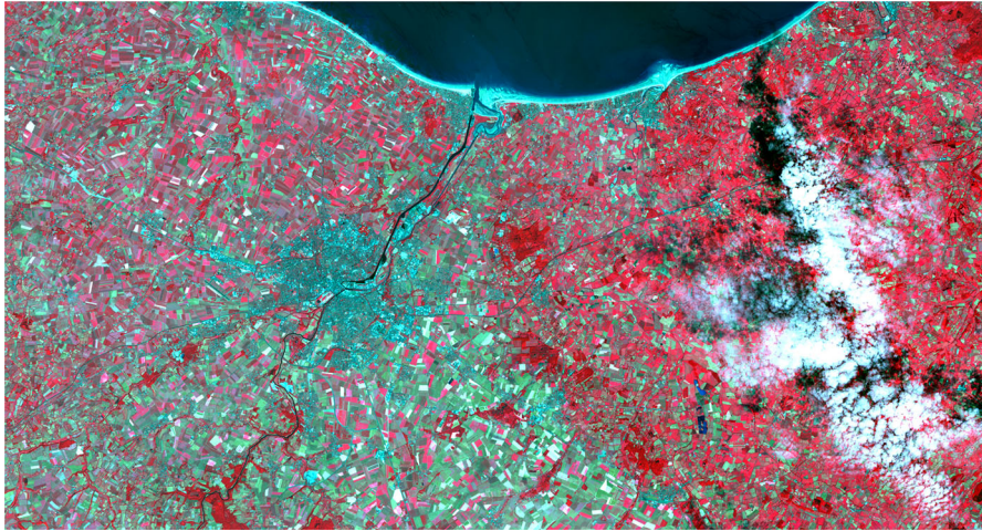
Fig. 9 Landsat-8 image taken on the 17th of July 2013—red displays near-infrared, green displays red and blue displays green (traditional false-color composite). Contains USGS/NASA Landsat Program data © 2013 processed at level 2A by CNES for THEIA Land data centre (Color figure online)
