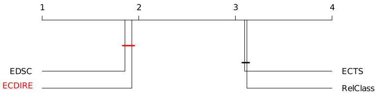
Fig. 7 Results from statistical tests for earliness. The ranking is issued from the Friedman test and shows the goodness of the methods from better to worse ( left to right ). The bold lines show the results issued from the Holm procedure, and joins pairs of methods that do not yield statistically significant differences
