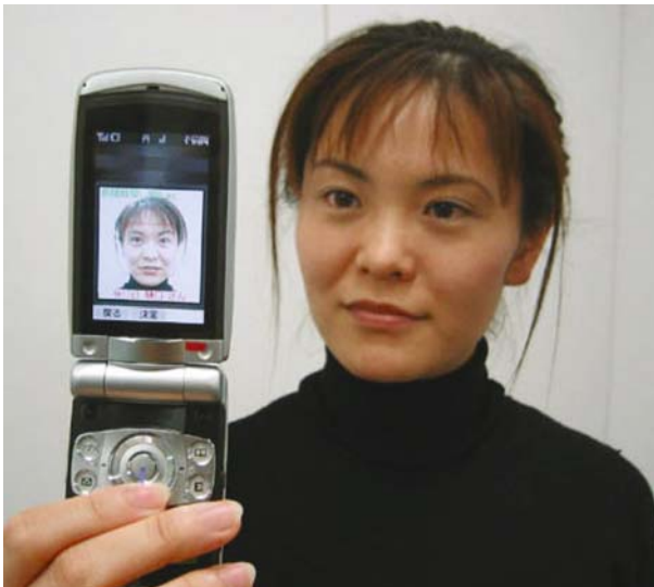
Fig. 12 Handset using OMRON OKAI vision sensor (Omron)
