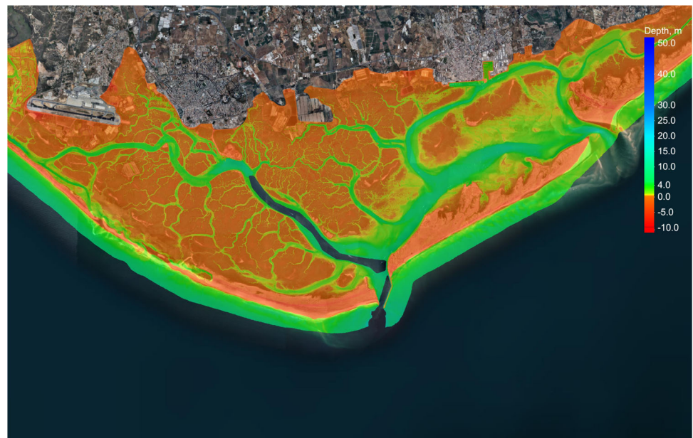
Fig. 6 LiDAR measurements of the bathymetry in the Ria Formosa lagoon [14, 39]
