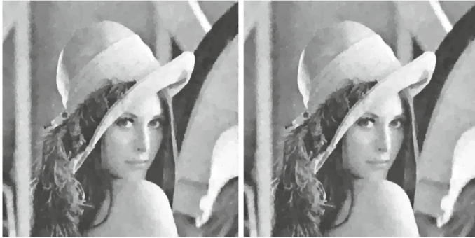
Fig. 7 TV problem for the test image Lena, which was contaminated with Gaussian noise with variance \sigma = 0.02 . (Left) image denoised with PMM. (Right) image denoised with ADMM. The image was denoised using \zeta = 30 and \rho = 1.8
