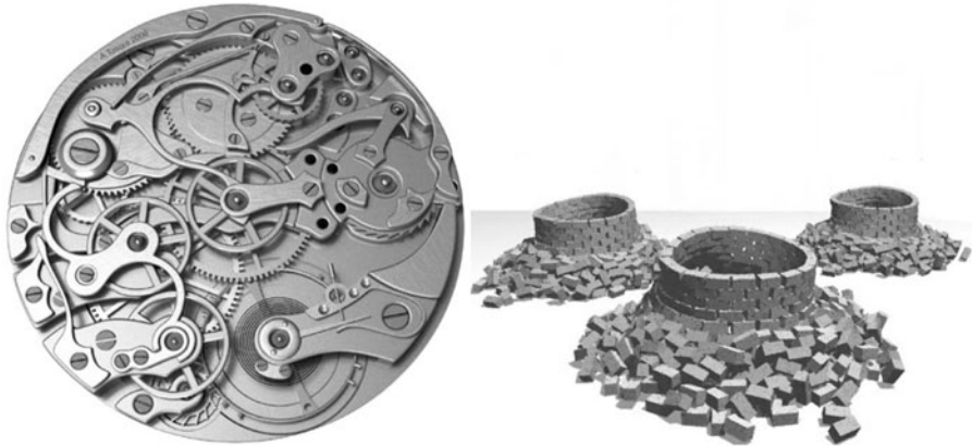
Fig. 1 Examples of multibody systems with many unilateral contacts
