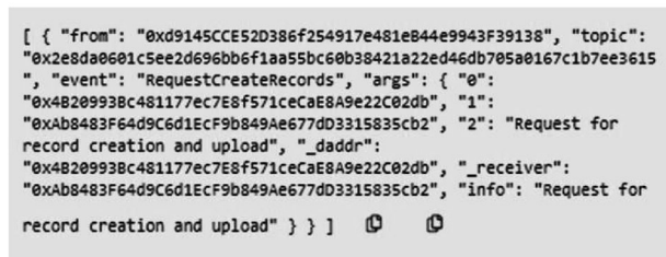
Fig. 5 Event log detail of Doctor Account request to create and upload records
