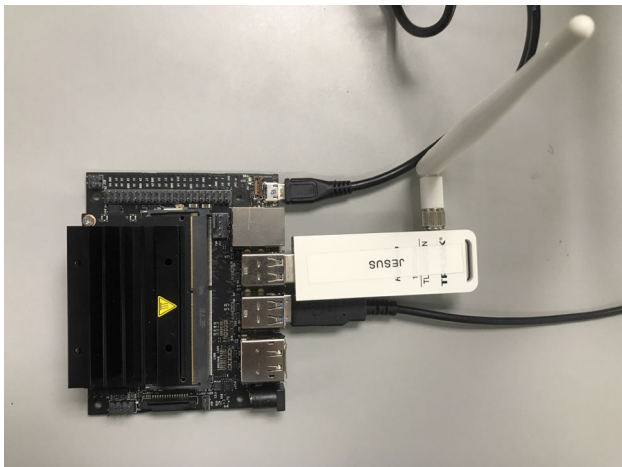
Fig. 3 NVIDIA Jetson Nano [24] used for the analysis of the EMG signals in real-time
