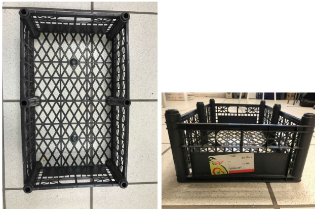
Fig. 6 Box used for the testing activity. The box size is 50x30x13 cm 3
