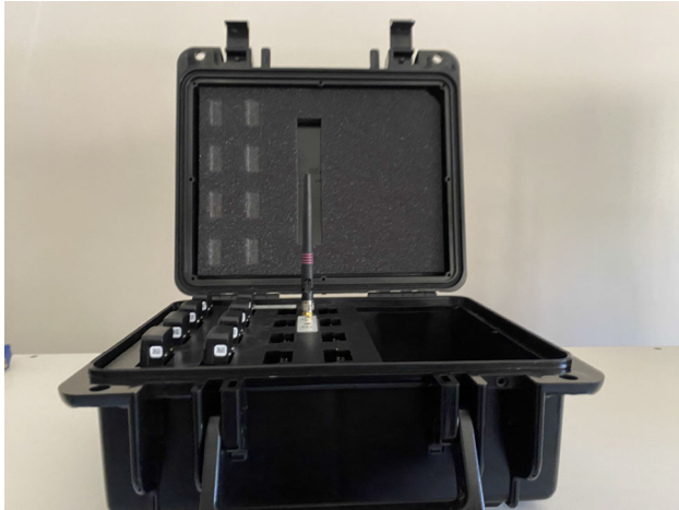
Fig. 2 Trigno wireless system [23] for EMG signals collection. The wireless sensors allow taking data in working environments like manual handling loads without affecting the activity of workers
