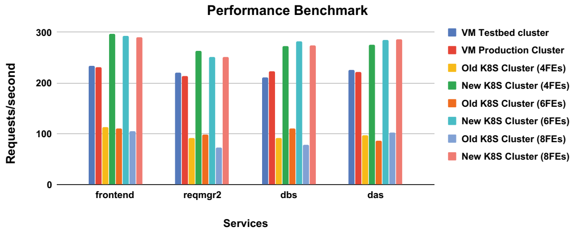
Fig. 10 The performance benchmark results in the form of requests/s (y-axis) of some of the commonly used CMSWEB services (x-axis) for various clusters (i.e. VM production cluster, VM testbed cluster,
