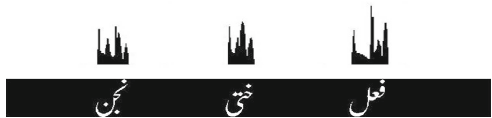
Fig. 10 Vertical projection profile for ligature segmentation
