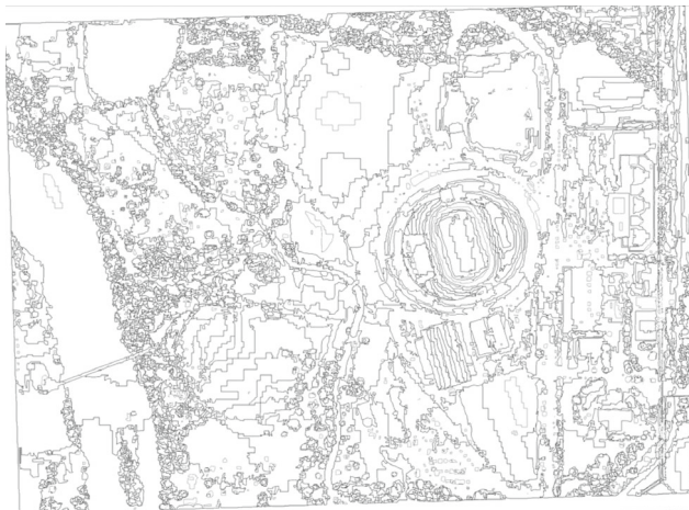
Fig. 8 Contour extraction from the height map of Fig. 7b.
