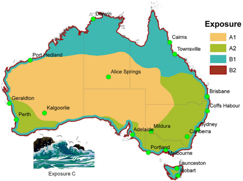
Fig. 2 Environment exposures of concrete structures in Australia
