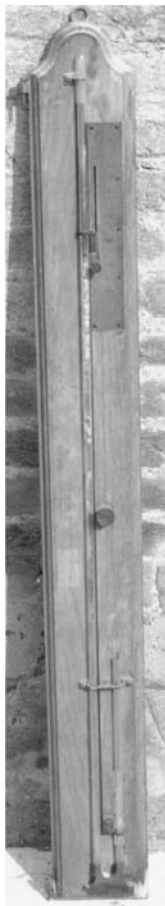
Figure 3. Siphon barometer with shape similar to the Gay Lussac type, still preserved at the Specola.
