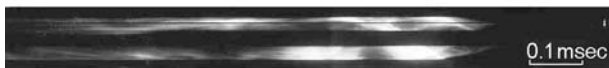
Fig. 6. Typical photographic record of forced initiation of detonation in a hydrogen–air mixture: the central window is closed; combination of injectors F2/A2, d_2 = 70 mm, H = 10 mm, at the moment of initiation (bright flash at the beginning of the record), P_c = 17 \cdot 10^5 Pa at the point R_c = 70 mm; \phi = 1.2 ; E_i = 0.33 J.
