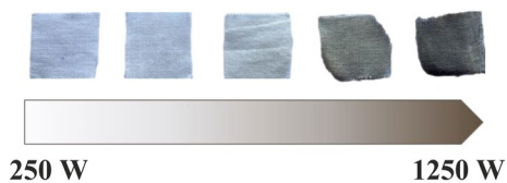
Fig. 6 External changes in the cotton fabric sample with an increase in RF power
