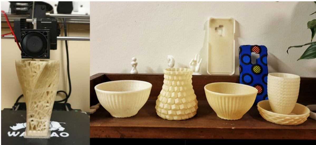
Fig. 13 FDM 3D printed items using PLA/CNF bionanocomposite filaments
