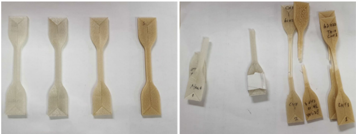
Fig. 16 Tensile test specimen of 6Neat, 6NeatTA10, TA10CNF1% and TA10CNF3% before (left) and after (right) uniaxial tensile analysis
