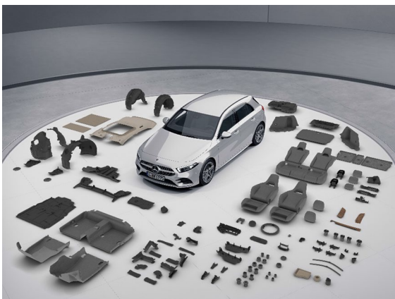
Fig. 8 Various natural fibre composite components of Mercedes-Benz A—class (Monteiro et al. 2010)
