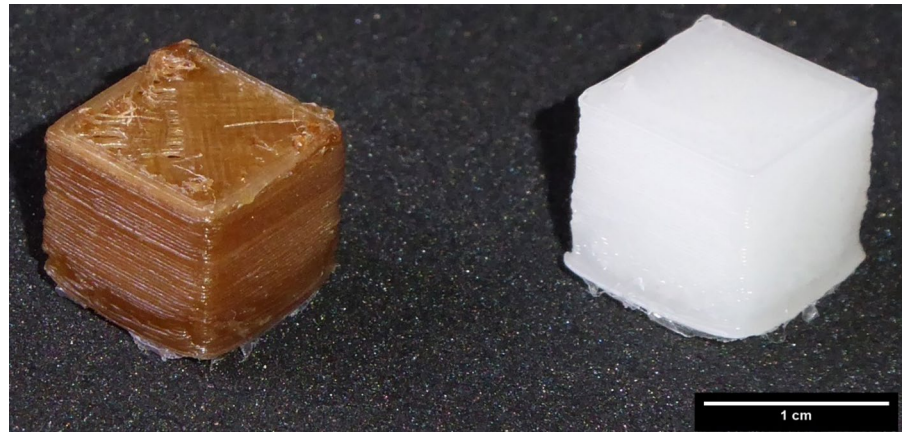
Fig. 7 picture of cubes 3D-printed respectively with a composite of CFPSA(10%)@HDPE (left) and with pure HDPE (right)
