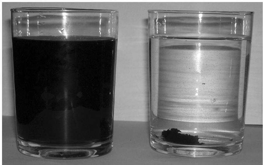
Fig. 1 Dispersion of activated carbon (AC) tablets in water. Left—AC tablet (0.22 g) modified by 0.018 g cellulose Na-sulfoacetate, right—a non-modified traditional tablet with starch as a binder
