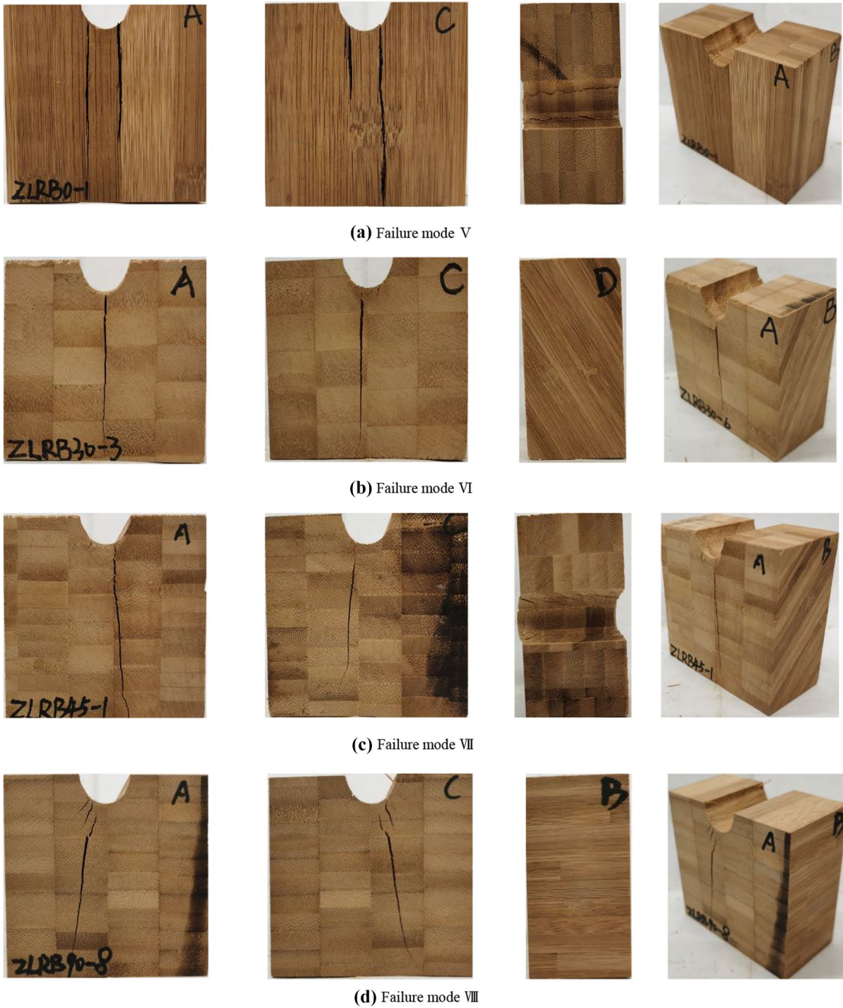
Fig. 6 Failure mode of class B specimen
