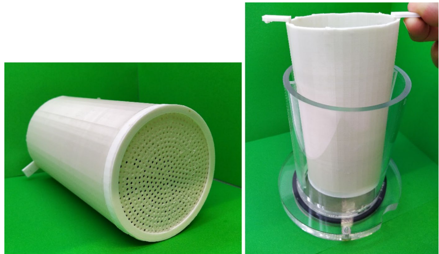
Fig. 3 The cylinder with perforated bottom was used to add MNFC suspension for multilayer forming
