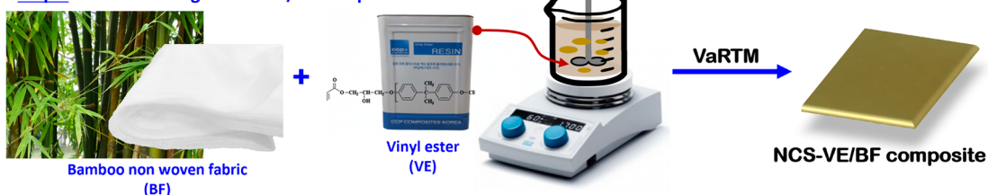
Scheme 1 Chemical reaction process for synthesis of NCS and scheme of manufacturing of NCS–VE/BF composites
