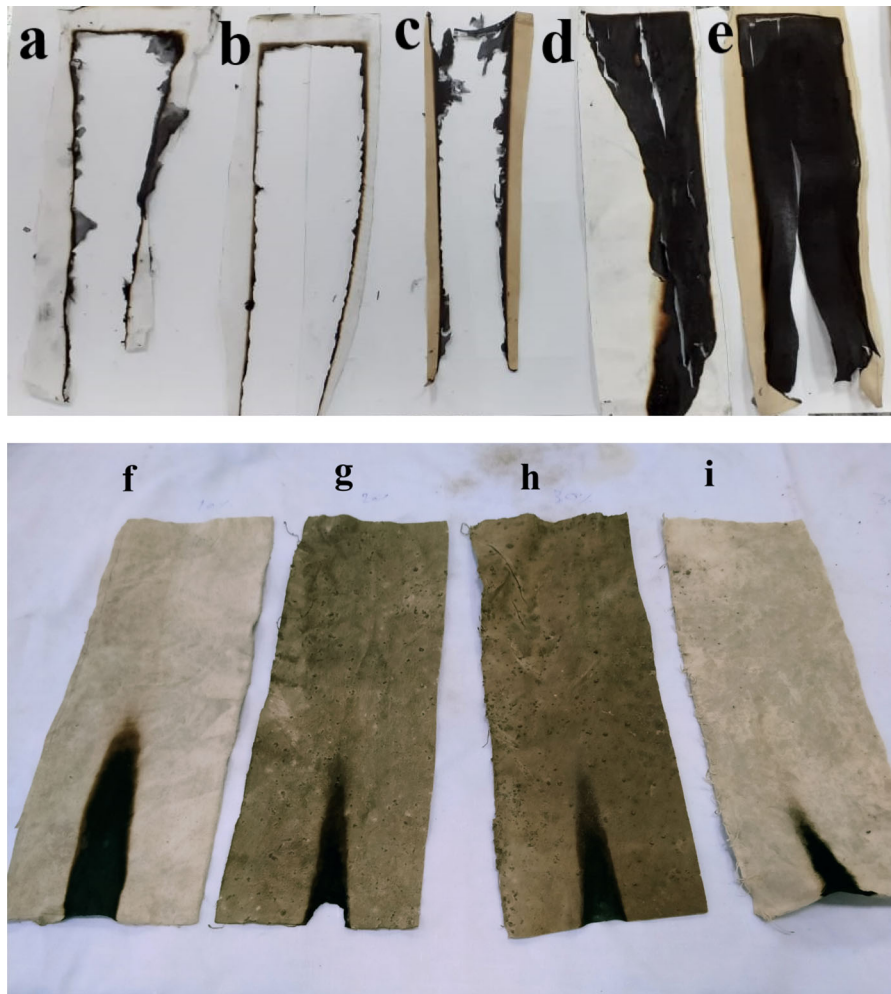
Fig. 4 Digital photographs for a control sample; b C1; c C2; d C3; e C4; f C5; g C6; h C7 and i C8 samples after the vertical burning test
