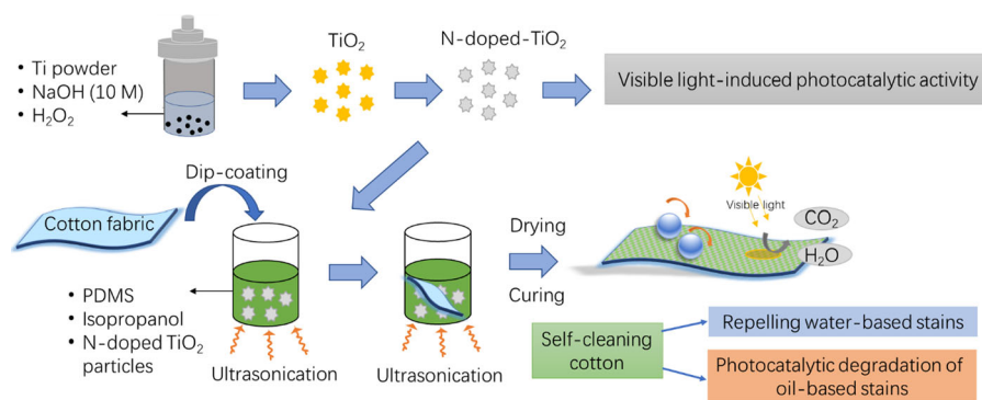
Fig. 1 Schematic illustration of preparing method of self-cleaning cotton fabrics
