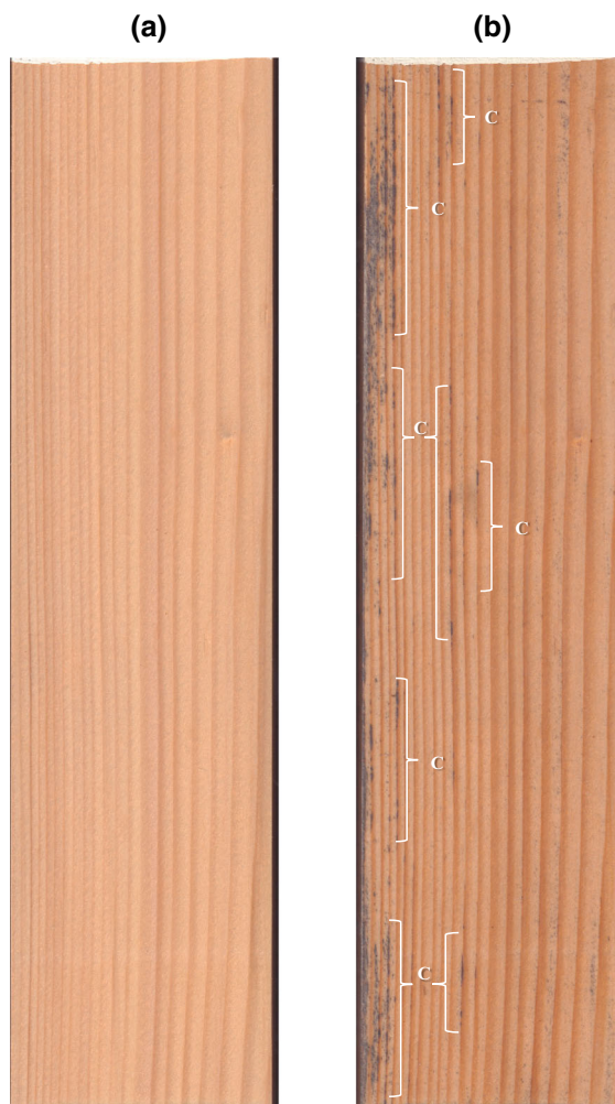
Fig. 5 Comparison of an exemplary specimen (BB-030-bp) as prepared (a) and after outdoor exposure exhibiting strong cracking (C—cracked area) and significant infections with biotic factors (b)
