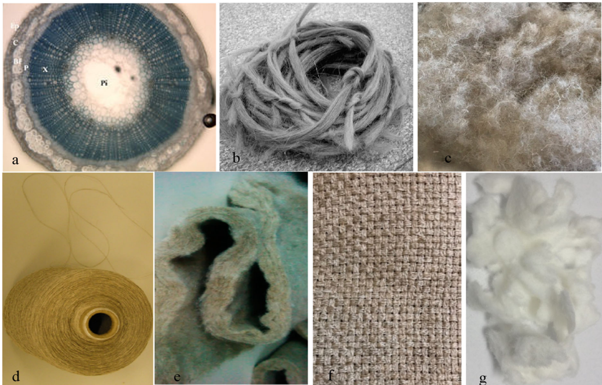
Fig. 9 a Flax stem cross-section showing locations of underlying tissues: Ep = epidermis; C = cortex; BF = bast fibers; P = phloem; X = xylem; Pi = pith. The stem of flax is around 2–3 mm in diameter; b the technical fiber is around 50–100 \mu\text{m} and consists of about 10–40 individual fibers in the cross-section. Individual fibers generally with diameters around 15–20 \mu\text{m} and lengths between 20–50 mm. The multiple
