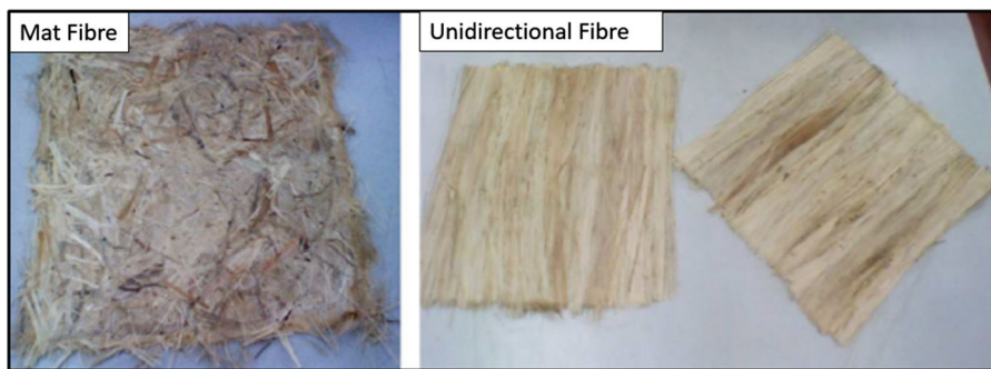
Fig. 3 Kenaf fibre mats and unidirectional fabrics (Fiore et al. 2015). Reproduced with permission from Fiore et al. 2015. Copyright 2015 Elsevier
