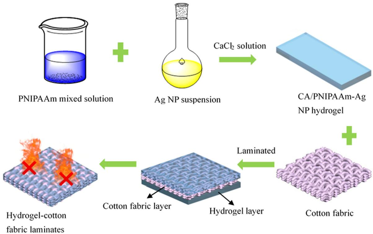
**Fig. 1** Schematic diagram of preparation of hydrogel–cotton fabric laminating
