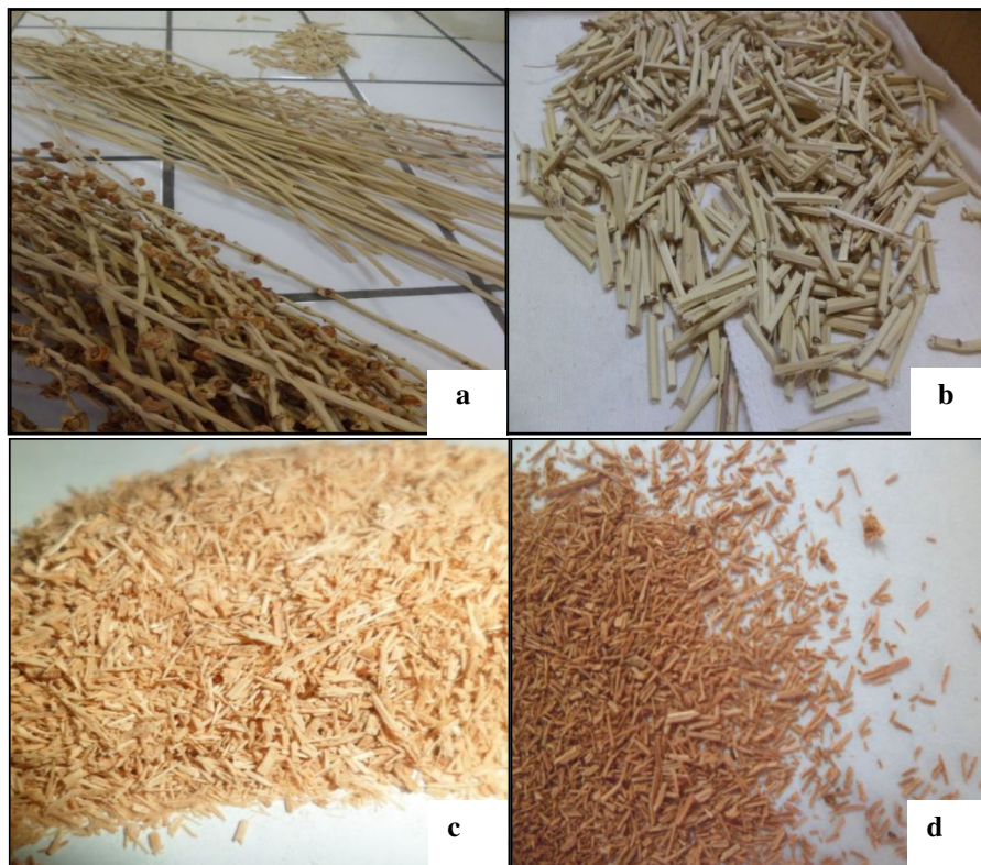
Fig. 1 Superficial morphology of palm date sawdust. a Stalks of palm date. b Cleaned, dried and cut stalks of palm date. c Untreated palm date sawdust. d Treated palm date sawdust
