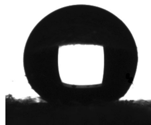
Fig. 5 Shape of a water drop on modified surface (M1P0)
