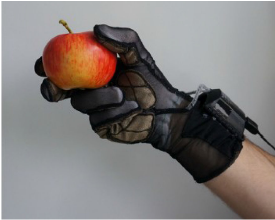
Fig. 5 Grasping an apple using the right hand tactile dataglove (Büscher et al. 2015). Copyright (2015) Robotics and Autonomous Systems, ELSEVIER
