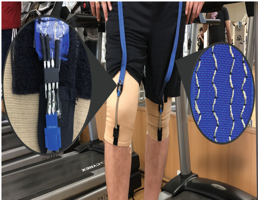
Fig. 1 The wearable textile sensing system for lower limb motion monitoring (Ozlem et al. 2019). Copyright (2019) Springer Nature Switzerland AG
