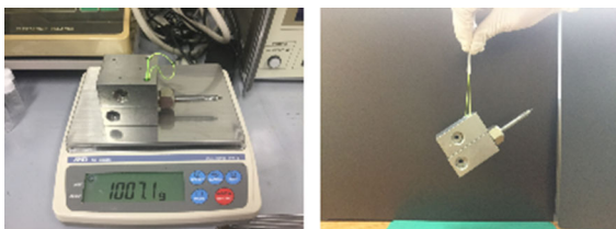
Fig. 2 Pictures of a weight of \sim 1 kg (left) and 2 wt% CNF-M/PVA/borax gel that lifts the weight (right)
