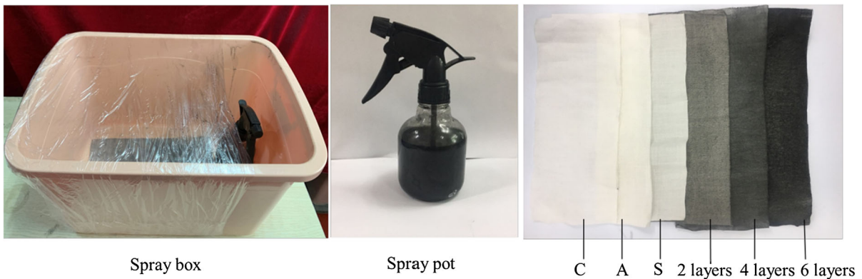
Fig. 3 Photographs of a spray box, a hand spray pot and treated ramie fabrics
